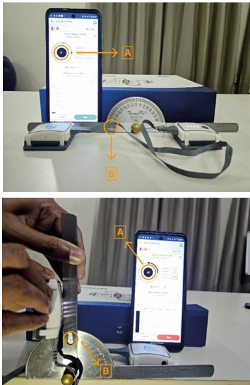
Figure 5: The Pheeze app view of recording the ROM data and verification by gold standard method. (a) Pheeze app and Goniometer are showing 0 degree in angle, (b) Pheeze app and Goniometer are showing 90 degrees in angle
