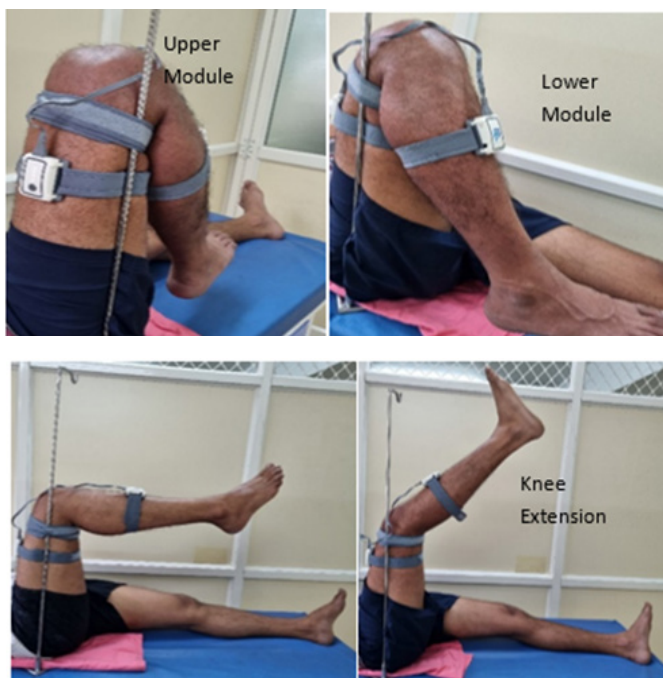
Figure 6: Upper and lower module placements
