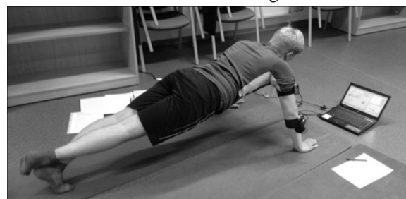
Figure 2: Push-up study training setup: The subject wears the two inertial sensors on the left or right arm. The VC is running on the notebook in front of the subject giving a visual (changing elbow angle) and auditory feedback (achieving the given threshold, 90° elbow angle).
