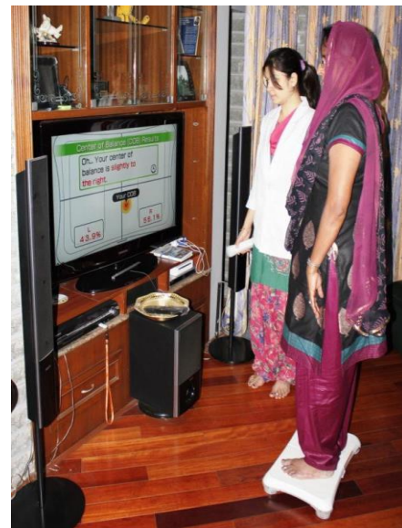
Figure 2: Subject standing with eyes open on WBB and weight distribution displayed on screen with centre balance.
