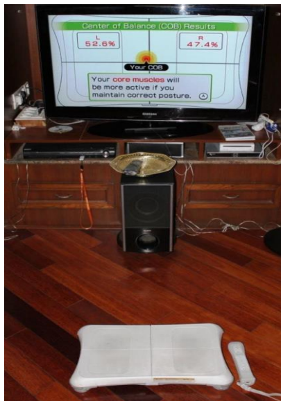
Figure 1: Showing WBB, Wii remote and screen displaying the percentage of weight distribution on right and left leg.
